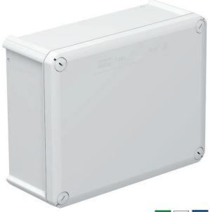
The junction boxes are made of a thermoplastic polypropylene polymer with closed side walls. This means that the required openings can be made wherever they are required. EDK plug-in seals or cable glands with locknuts can be inserted in these openings, to allow cable insertion. The junction boxes can be mounted on mounting plates in the openings on the floor using steel
