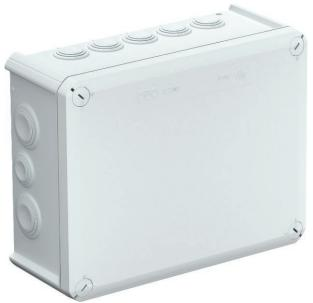
All the T series junction boxes are UV-resistant. They are made of a thermoplastic polypropylene plastic with plug-in seals made of ethylene vinyl acetate (EVA). This plastic is soft, which means that it is malleable. This allows installation of cables through the 9 x M25  $\,$
