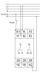
Range 1A, supply voltage 230V a.c. and fault latch
